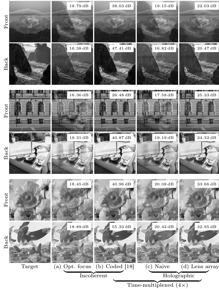
Fig. 2: More complex depth-varying projectors. (a) We show an optimized version of a focus-tunable lens/high-speed projector, where the patterns projected for each distance are jointly optimized. This increases performance over Fig. 1(b), but still does not match Fig. 1(d). (b) We demonstrate a 4\times time-multiplexed coded aperture projector [18], which significantly increases performance over the single aperture/display pattern case. (c), (d) We demonstrate 4\times time-multiplexed versions of a naive holographic system and an étendue-expanded version with the same field-of-view. Time multiplexing mildly improves performance for these holographic systems. In general, while time multiplexing is beneficial, there are practical challenges towards implementation, like increased bandwidth and lower framerates. Furthermore, time-multiplexed coded aperture requires an additional SLM, and will be significantly darker than a holographic approach thanks to the requisite light attenuation.
