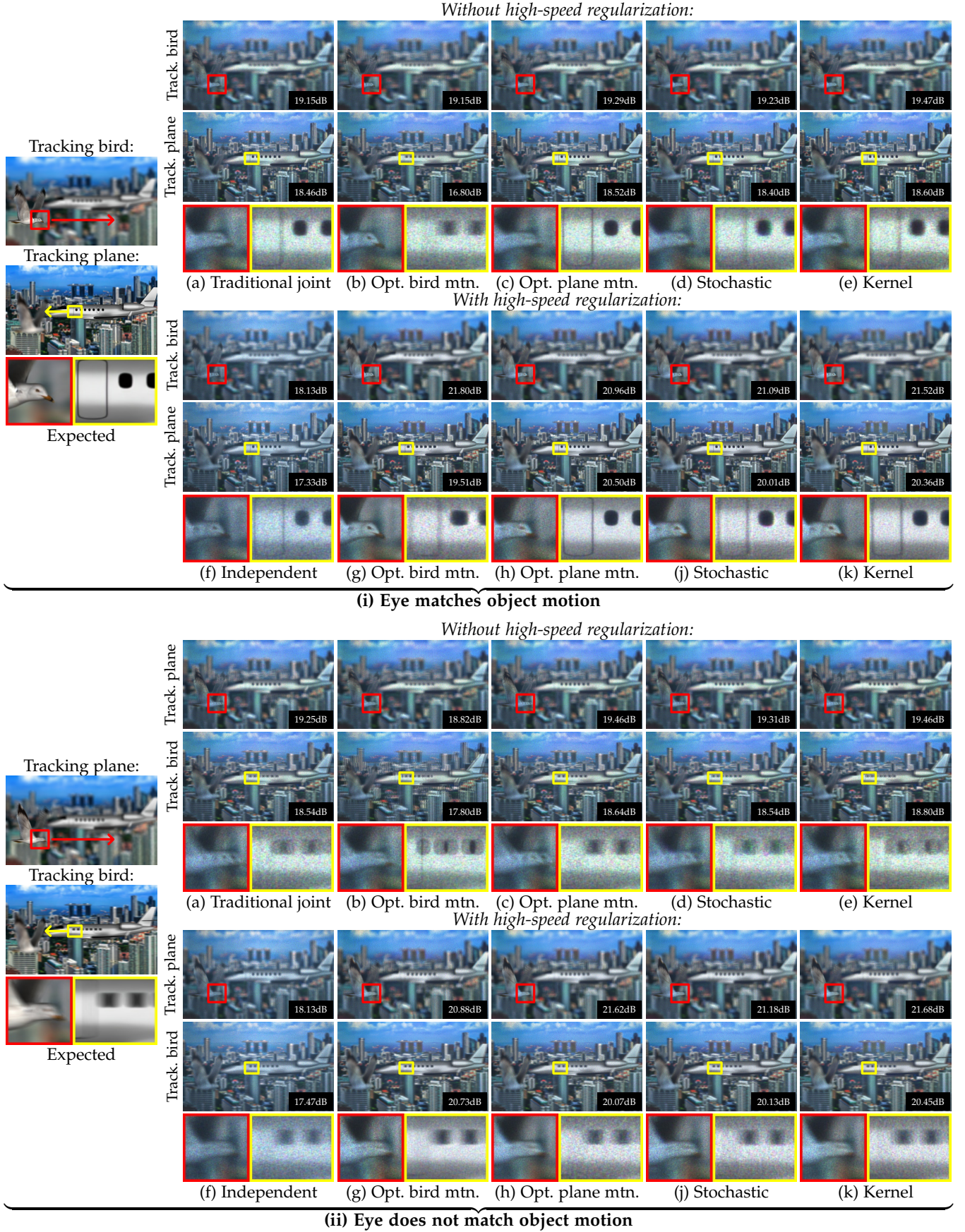
Fig. 9. Low compute visualization (simulation, full). We test our approach with just 4 iterations of gradient descent instead of 500. Our proposed framework is again able to mitigate sample-and-hold blur as well as strobing effects. Unlike higher-compute settings, the kernel-based approach slightly outperforms the stochastic approach, as insufficient iterations are performed to cover the entire space of possible motions under the stochastic methodology.
